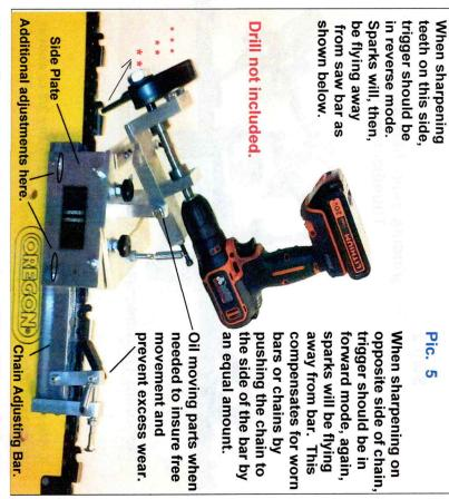
\*Note: For smaller chain saw bars, such as 3/8 or 404, mounting bolts on Side Plate should be in lower set of bolt holes in Chain Adjusting Bar. Position Chain Adjusting Bar even with front of Side Plate, as a point of reference. Further adjustments can be made within the slots if needed.
