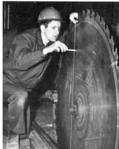
Figure 46. Check saw for plumb by dropping a bob alongside and measuring at various places along the line.
