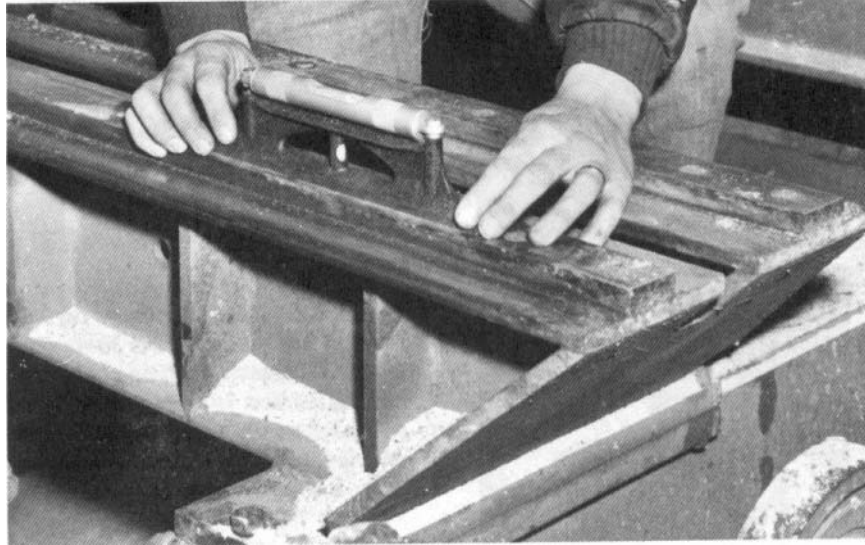
Figure 49. – Check the headblock base with a high quality machinist's level.
