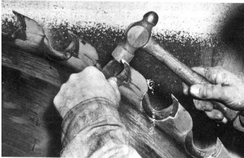
Figure 32. — Seat shanks in place by striking them with a firm blow.
